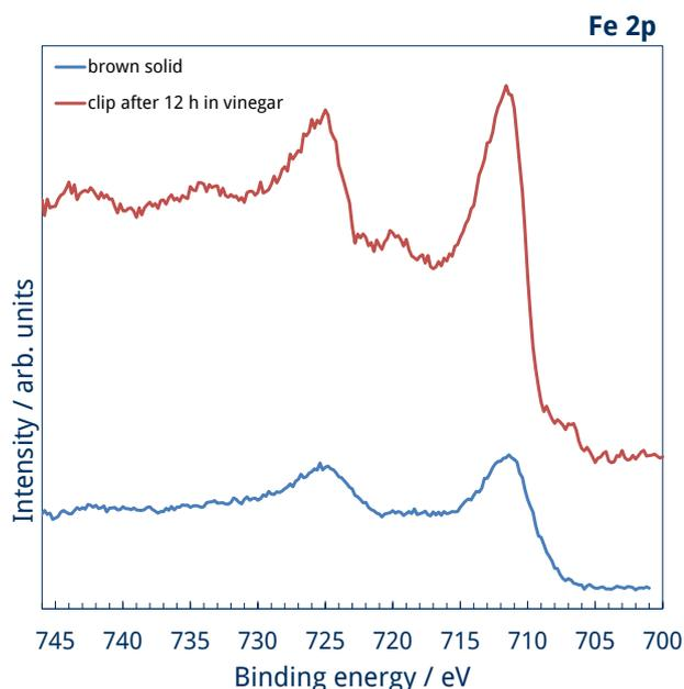
**Fig. 8 Fe 2p spectra of a corroded paper clip after 12 h immersion in vinegar (red) and the brown solid (brown).**
