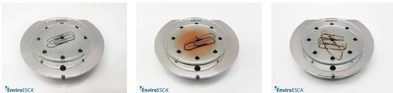
Fig. 1 Paper clip immersed in a concentrated vinegar solution (25 % acid) at different stages of corrosion (left and middle) and after complete evaporation (right) of vinegar solution.
