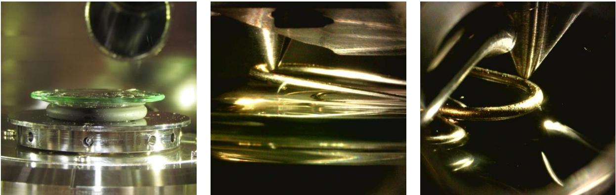
Fig. 5 Paper clip immersed in a concentrated vinegar solution (25 % acid) in the sample environment (left) and during live acquisition at 9 mbar under the nozzle (middle, right) of EnviroESCA.
