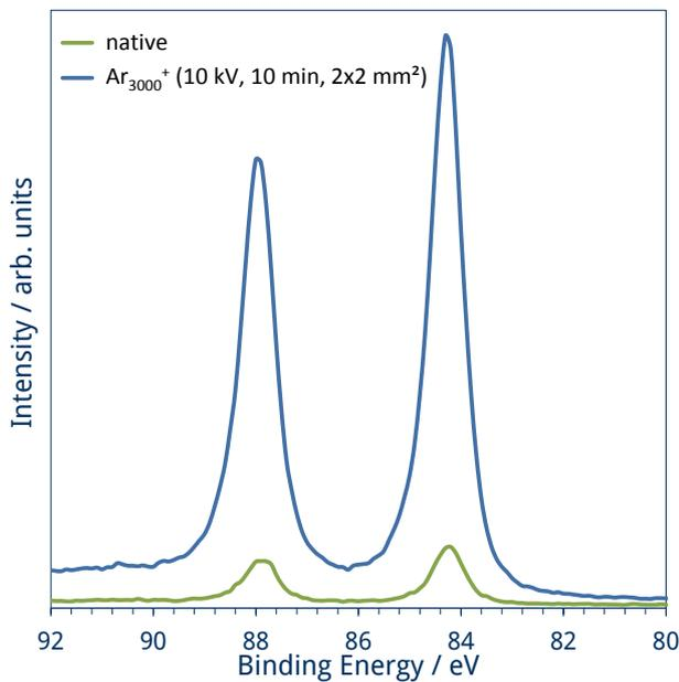
Fig. 6. Au 4f core-level spectra of a gold sample before (green) and after (blue) GCIB sputtering (2x2 mm<sup>2</sup> area,  $Ar_{3000}^+$  10 kV, 10 min)
