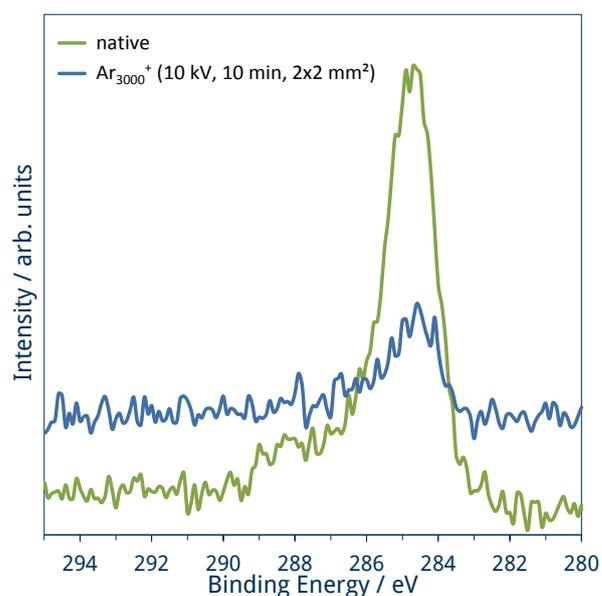
Fig. 5. C 1s core-level spectra of a gold sample before (green) and after (blue) GCIB sputtering (2x2 mm<sup>2</sup> area,  $Ar_{3000}^+$  10 kV, 10 min)
