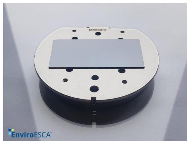
Fig. 1 Sample of an ultra-thin organic film on silicon used for sputter depth profiling with argon gas clusters
