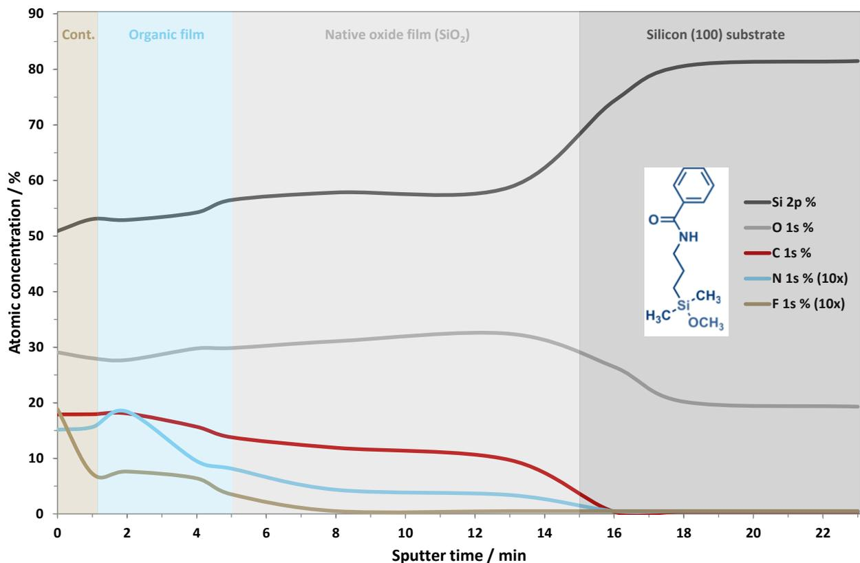
Fig. 7. XPS sputter depth profile of an ultra-thin DMSPPA film ( $1.4 \pm 0.5$  nm) on a SiO<sub>x</sub>/Si(100) surface. The chemical structure of DMSPPA is given as inset. The sample was sputtered using an argon GCIB with  $Ar_n^+$  clusters first at 5 kV (4 min  $Ar_{3000}^+$ , 9 min  $Ar_{2000}^+$ , 1 min  $Ar_{1000}^+$ ) then at 10 kV ( $Ar_{2000}^+$ ). A raster size of 5x5 mm<sup>2</sup> was used. Elemental compositions are given in atomic percent.
